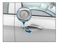
Insert the key in the slot and turn it clockwise to lock and anticlockwise to unlock the door.
