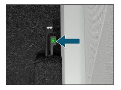
6. Open the protective cap on charging inlet.
