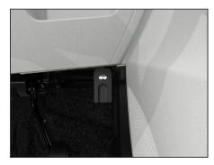
Raise the bonnet slightly and with your finger slide the secondary lock lever located under the bonnet centre to the left side.
