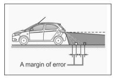
When any part of the vehicle sags due to the number of passengers or the distribution of the load, there is a margin of error between the fixed guide lines on the screen and the actual distance/course on the road.
