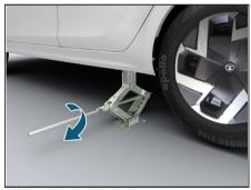
Lifting the rear wheel using jack
