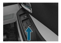
When switch (5) is pressed, amber light turns 'OFF'. The individual switches provided on rear and front passenger door can be operated. It can also be operated from the switches on driver's arm rest.
