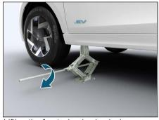
Lifting the front wheel using jack
