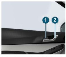
All the doors can also be locked from inside by pressing knob on driver door and independently on other doors respectively.
