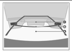
Visually check the surroundings and the area behind the vehicle. On the screen, it appears that a truck is parked at point B. However, in reality if you back up to point A, you will hit the truck. On the screen, it appears that A is closest and C is furthest away. However, in reality, the distance to A and C is the same, and B is further away from A and C.
