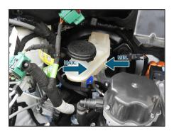
The level of the brake fluid should be between the 'MIN' and 'MAX' marks on the side of the brake fluid container. If the level falls below the 'MIN' mark, add recommended brake fluid.
