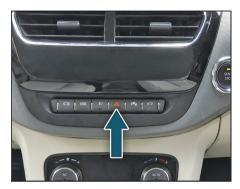
Press the hazard warning switch to activate the hazard warning. All the turn signal lamps will flash simultaneously. To turn OFF, press the switch again.
