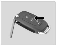
Press and hold approach light button for few sec until the trunk lid is unlock.
