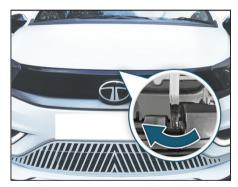
Lift the bonnet up. Pull the bonnet stay rod from its clip and engage the free end into the slot.
